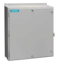
Non-reversing motor starter, Size 3, Three phase full voltage, Solid-state overload relay, OLRelay amp range 25-100A, 24VAC 50-60HZ coil, Non-combination type, Enclosure type 12, Dust/drip proof for indoors, Extra-wide enclosure
