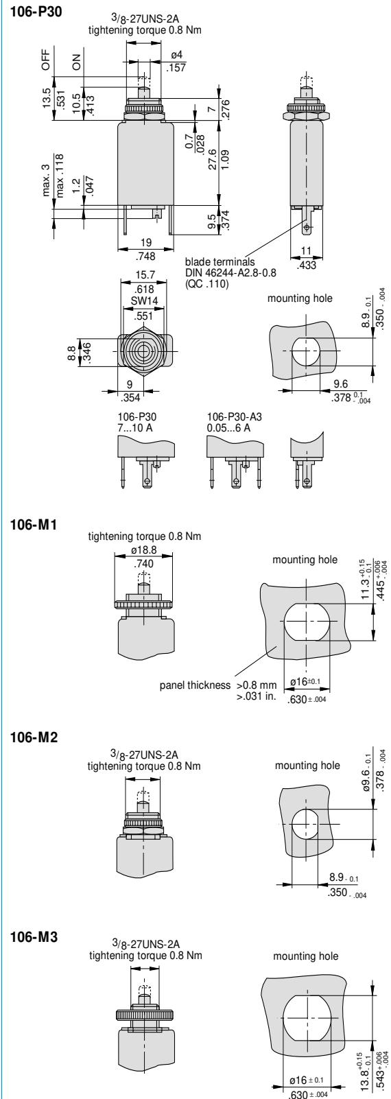
This is a metric design and millimeter dimensions take precedence ( $\frac{\text{mm}}{\text{inch}}$ )
