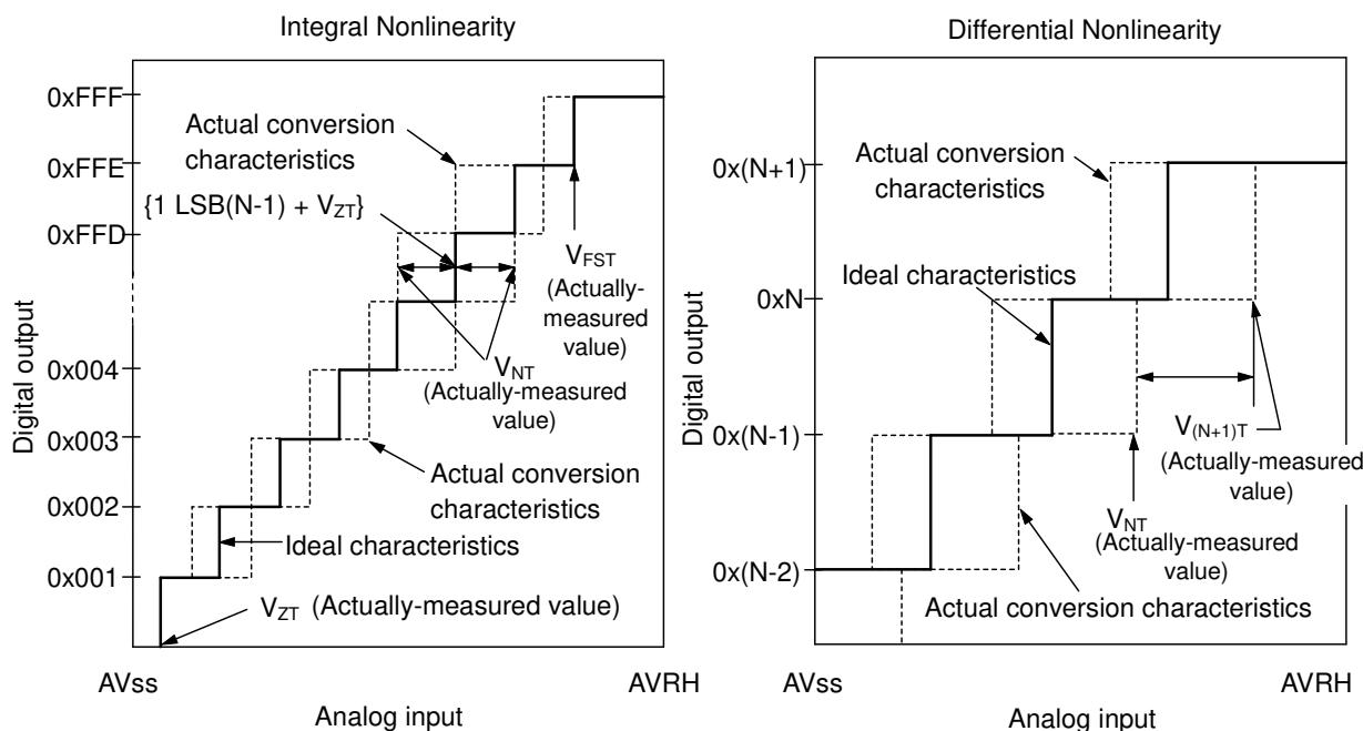
$$\text{Integral Nonlinearity of digital output } N = \frac{V_{NT} - \{1\text{LSB} \times (N - 1) + V_{ZT}\}}{1\text{LSB}} \quad [\text{LSB}]$$
