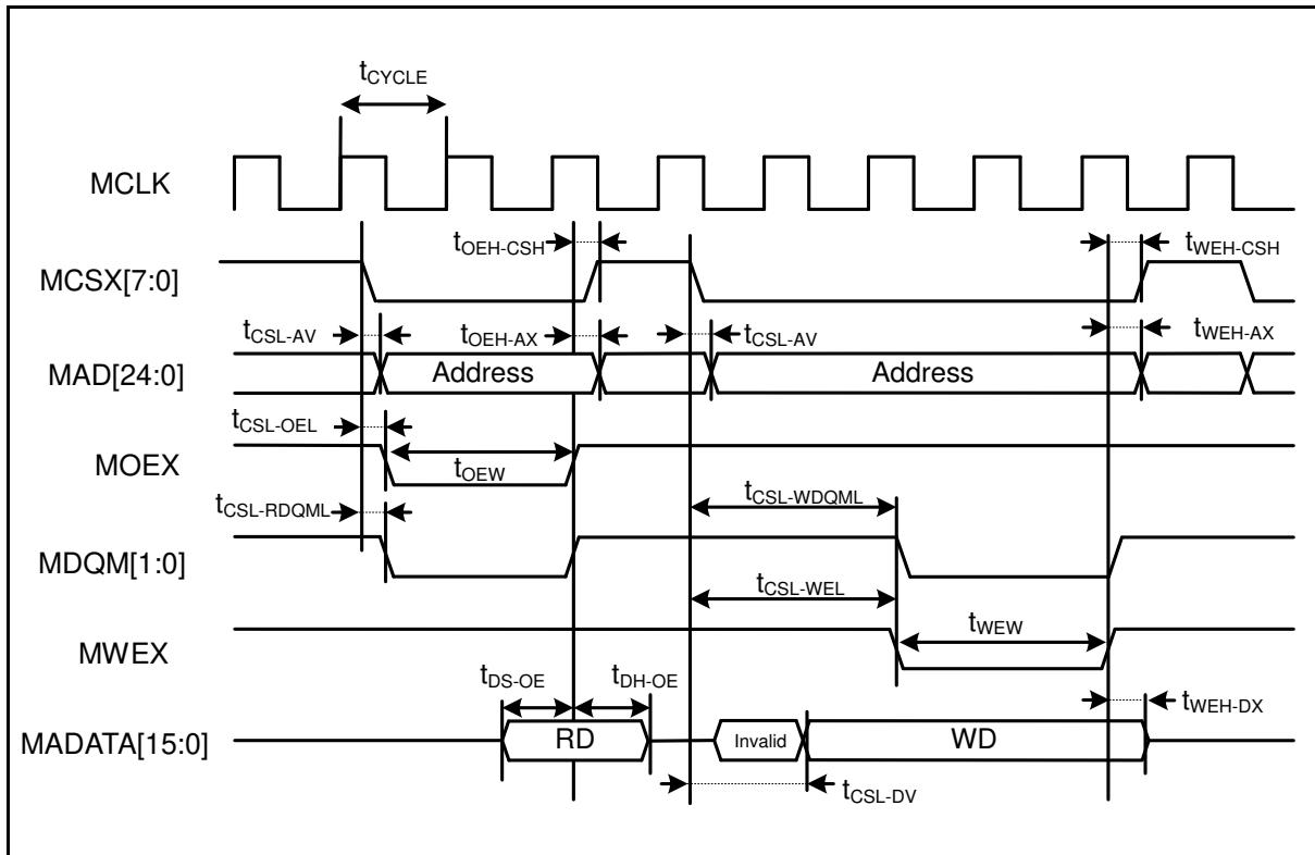
**Separate Bus Access Synchronous SRAM Mode**
