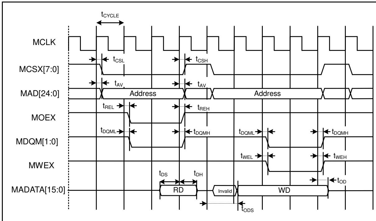
**Multiplexed Bus Access Asynchronous SRAM Mode**
