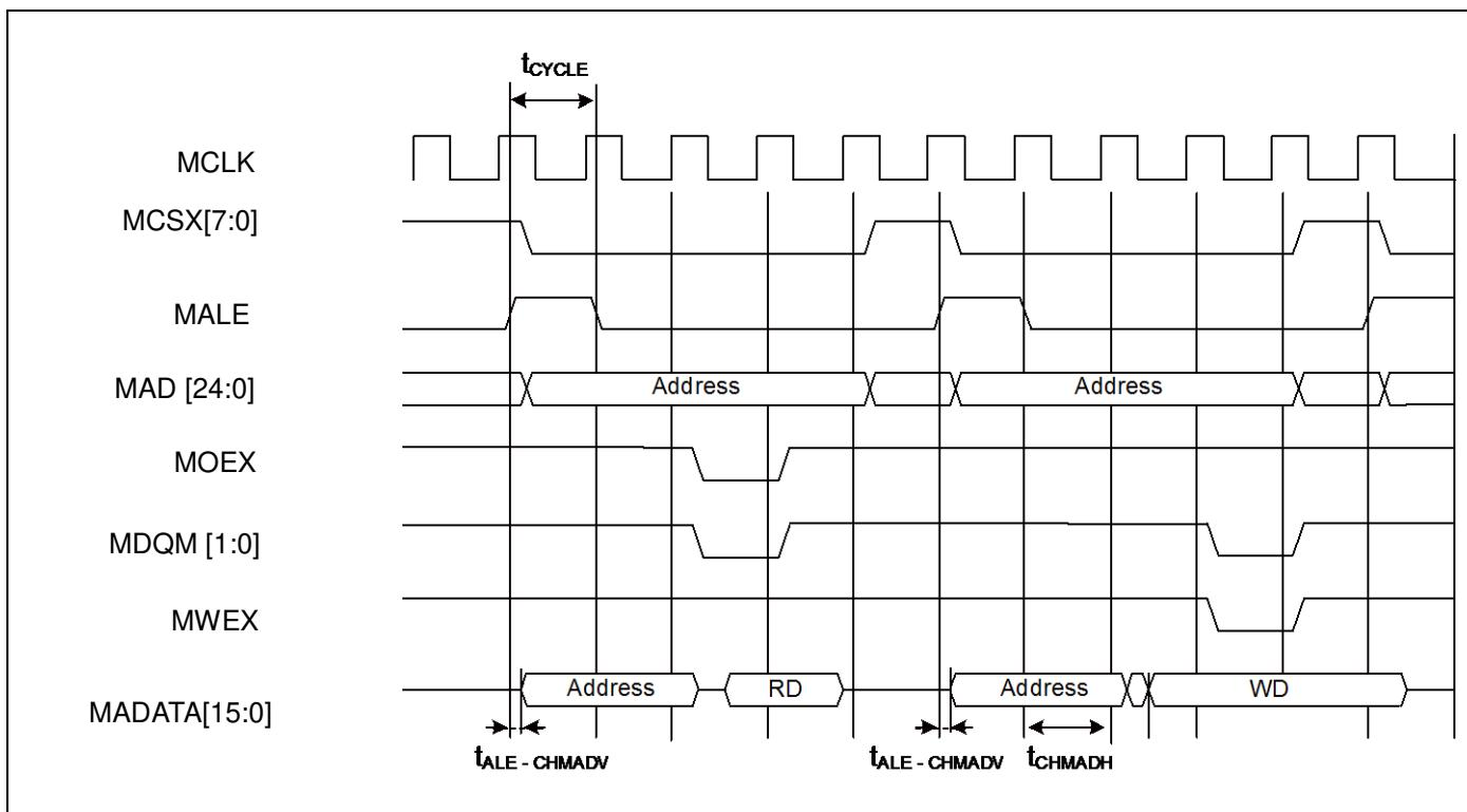
**Multiplexed Bus Access Synchronous SRAM Mode**
