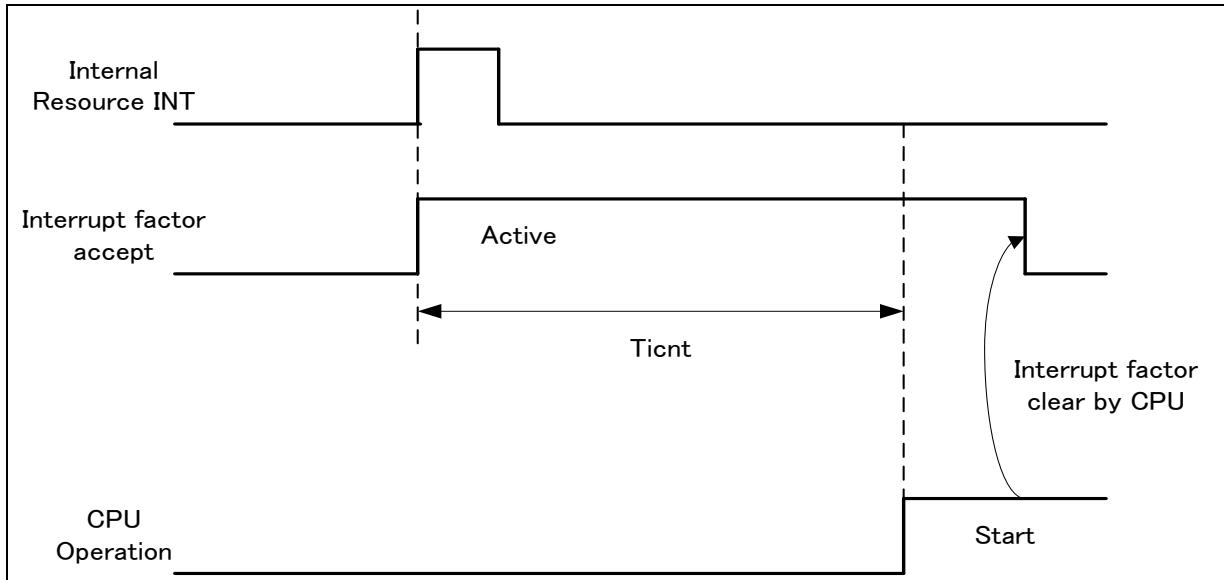
\*1: Internal resource interrupt is not included in return factor by the kind of Low-Power consumption mode.
