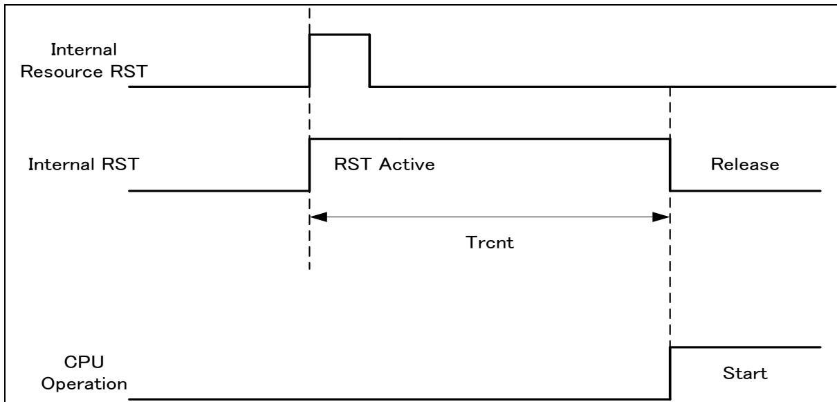
\*1: Internal resource reset is not included in return factor by the kind of Low-Power consumption mode.
