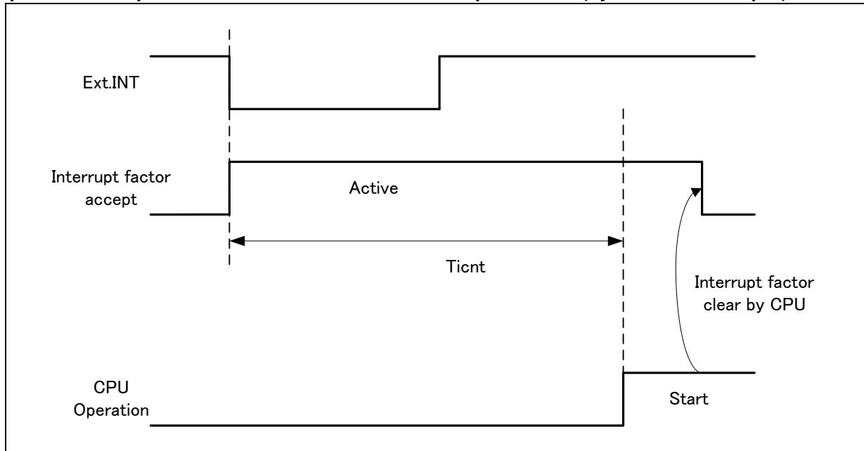
\*1: External interrupt is set to detecting fall edge.
