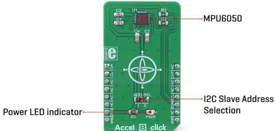
Three-axis gyroscope MEMS can be programmed to measure the rotation about each axis, in four different ranges of rotational speed (degrees per angle, DPS):  $\pm 250$ ,  $\pm 500$ ,  $\pm 1000$ , and  $\pm 2000$ . Three-axis accelerometer MEMS can be programmed to measure the acceleration along each axis, in four different acceleration ranges:  $\pm 2g$ ,  $\pm 4g$ ,  $\pm 8g$ , and  $\pm 16g$ . The user can select an optimal range for both properties, depending on the application requirements.
