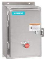
Non-reversing motor starter, Size 1 3/4, Three phase full voltage, Solid-state overload relay, OLR amp range 10-40A, Non-combination type, Encl. type 4X 304 S. Steel, Water/dust tight noncorrosive, Standard width enclosure
