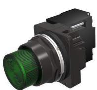
30mm BlackMax, Epoxy Coated Corrosion Resistant Complete Metal Unit Illuminated Indicator Light Full Voltage type, 24V AC/DC Super Bright LED Lamp, BA9s Plastic Lens, Green UL Listed, CSA Certified NEMA 1,3,3R,4,4X,12,13 & Automotive Standards
