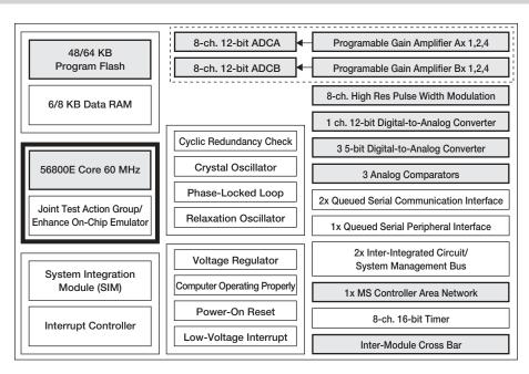
flexibility and compact program code, the MC56F825x/MC56F824x is well-suited for many consumer and industrial applications especially advanced power conversion and motor control.
