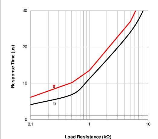
Testcondition: I<sub>C</sub>= 2mA; V<sub>CF</sub>= 2V; TA= 25°C
