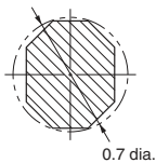
XC5E DIP terminal cross-section view
