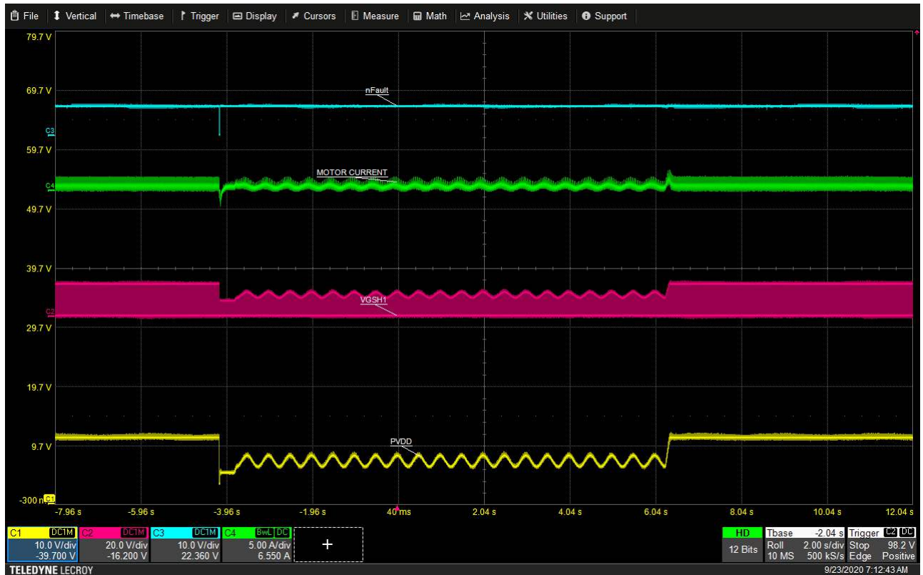
Figure 8-5. Driver PWM Operation During Cold Crank Pulse
