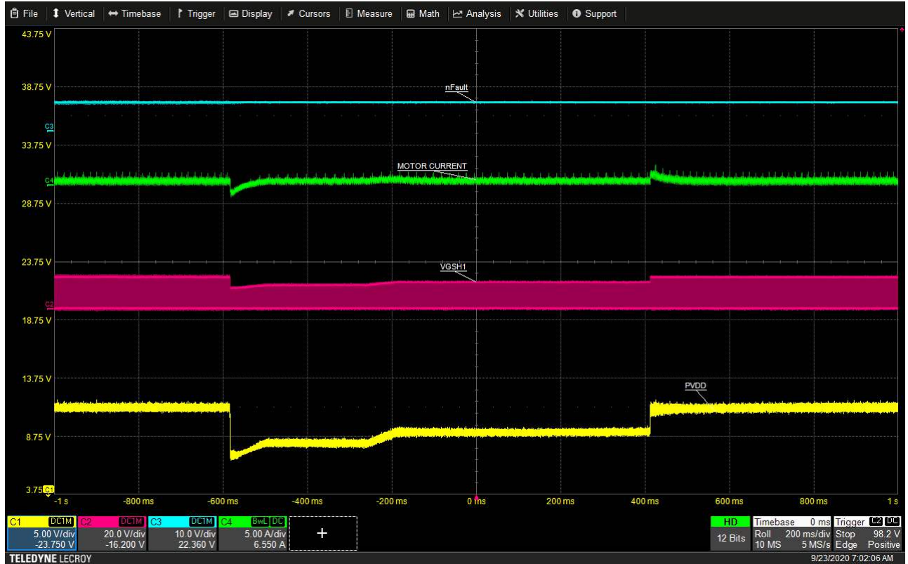
Figure 8-4. Driver PWM Operation During Warm Crank Pulse
