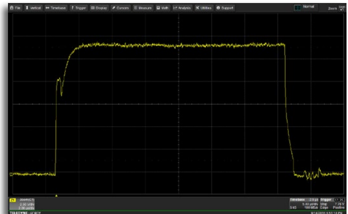
Current sinking into half-bridge phase in cascaded H-bridge – HVFO enables Miller effect to be observed clearly
