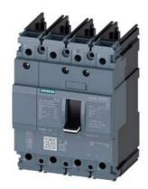
circuit breaker 3VA5 UL frame 125 breaking capacity class H 65kA @ 480V 4-pole, line protection TM210, FTFM, In=15A overload protection Ir=15A fixed short-circuit protection Ii=20 x In N conductor unprotected without connection
