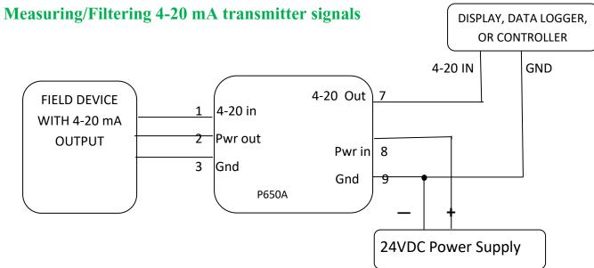
This unit is powered with 24VDC. Positive voltage on terminal 8 and common or ground on terminal 9 The unit will provide 24VDC power and ground for the field device when connected as shown
