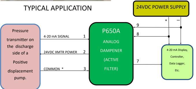
\* Common is not needed with 2 wire transmitters
