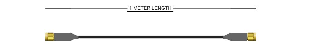
Connector A 132451 SMA Plug Straight Brass Gold + Heatshrink 50 Ohm LMR-240 Continuity/Hi-Pot Connector B 132451 SMA Plug Straight Brass Gold + Heatshrink
