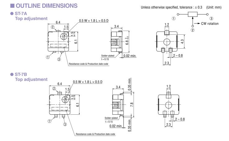
\* The ST-7 series has a different terminal arrangement from the ST-3 and ST-4 series. Pay attention to the location of terminals number 1 and 3. (Resistance decreases when the shaft is turned CCW.)
