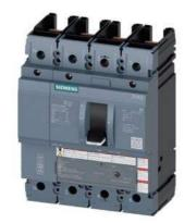
circuit breaker 3VA5 UL frame 250 breaking capacity class H 65kA @ 480V 4-pole, line protection TM230, FTAM, In=225A overload protection Ir=225A fixed short-circuit protection Ii=5...10 x In N conductor protection 100% without connection
