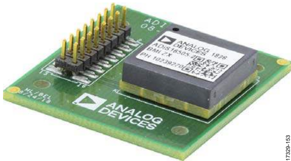
Figure 64. ADIS16507-2 Breakout Board (ADIS16505-2 Shown)
