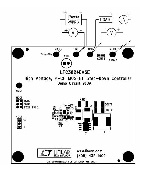
Figure 1. Proper Measurement Equipment Setup
