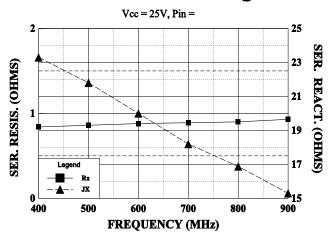
SERIES INPUT IMPEDANCE vs FREQUENCY
