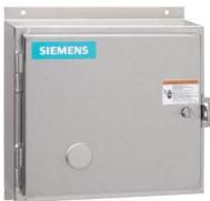
Reversing NEMA contactor Size 0 Three phase full voltage Contactor amp rating 18Amp 3 w 110-120/220-240VAC 60HZ coil Non-combination type Encl NEMA type 4X 304 S-steel Standard width enclosure
