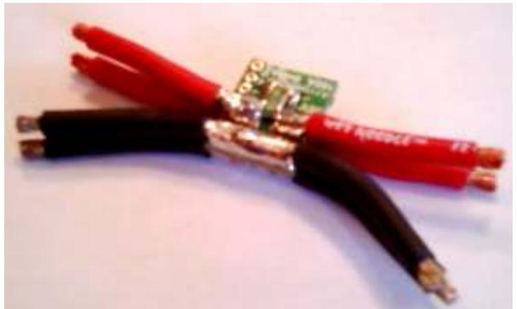
**180 Amp Sensor – Recommended Lead Arrangement**
