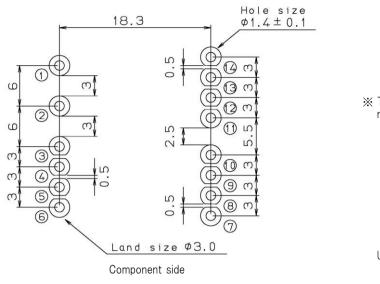
X The round pulling out figure is a pin numbering.
