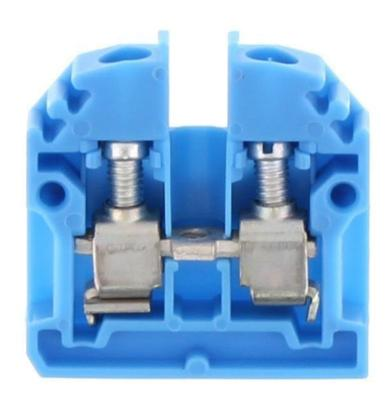
Feed-through terminal for direct mount, Screw connection, Mounting type: Mounting surface, Rated cross-section: 4 mm², Width: 6 mm, Colour: Blue
