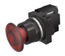
30mm BlackMax, Epoxy Coated Corrosion Resistant Complete Metal Unit Illuminated Push-Pull Operator Transformer type, 480V AC Incandescent Lamp Mushroom Head Cap Small 1 3/4" (44.5 mm) Plastic, Red 3 Position Momentary UL Listed, CSA Certified NEMA 1,3,3R,4,4X,12,13 & Automotive Standards
