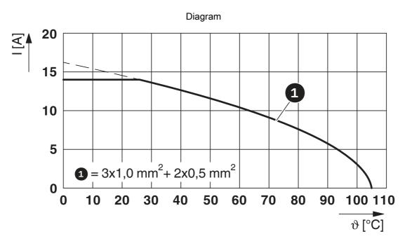
I = current strength,  $\vartheta$  = ambient temperature, 3x 14 A + 2x 2 A constant
