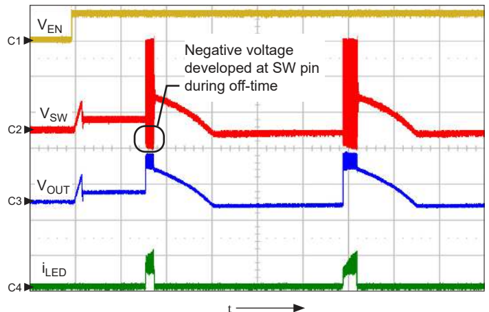
Figure 11: Startup waveform with a missing Schottky diode; shows Enable, V_{EN} (ch1, 5 V/div.), switch node, V_{SW} (ch2, 5 V/div.), output voltage, V_{OUT} (ch3, 5 V/div.), LED current, i_{LED} (ch4, 500 mA/div.), t = 100 \mu\text{s}/\text{div} .
