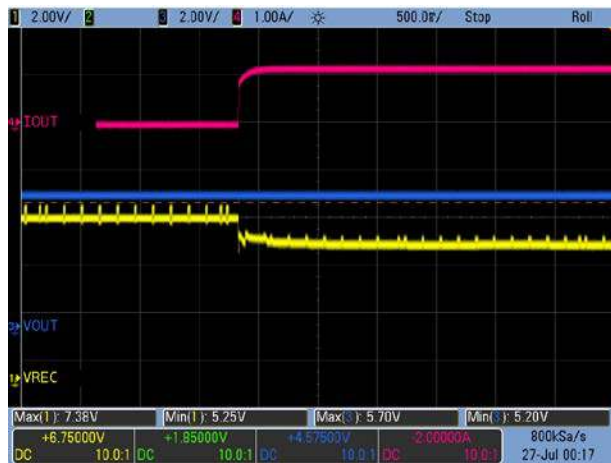
Figure 11. Load Transient: V OUT = 5V, 0A → 1.2A
