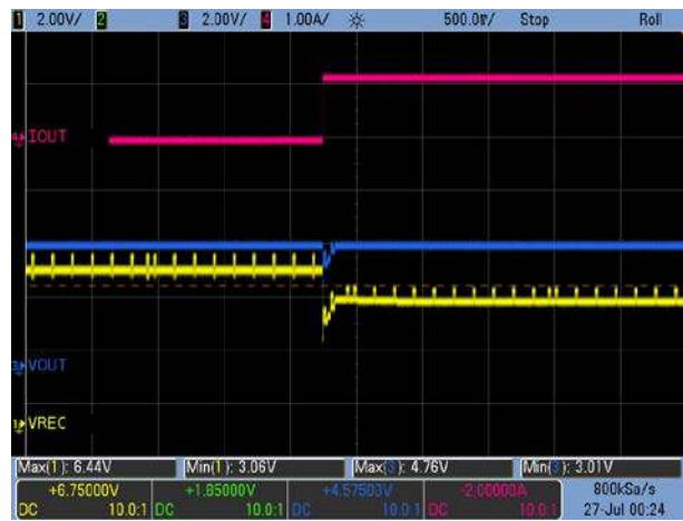
Figure 13. Load Transient: V_{OUT} = 4.5V, 0A \rightarrow 1.2A
