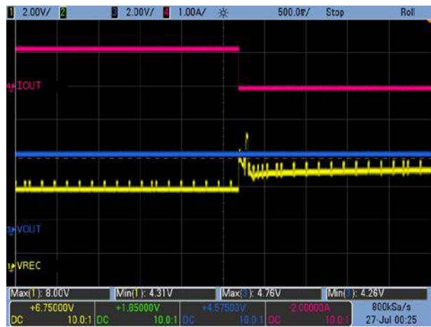
Figure 14. Load Transient: V_{OUT} = 4.5V, 1.2A \rightarrow 0A
