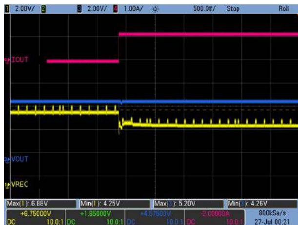
Figure 11. Load Transient: V OUT = 5V, 0A → 1.2A
