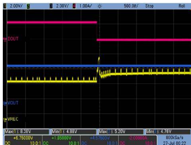
Figure 12. Load Transient: V OUT = 5V, 1.2A → 0A
