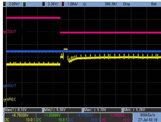
Figure 12. Load Transient: V OUT = 5V, 1.2A → 0A
