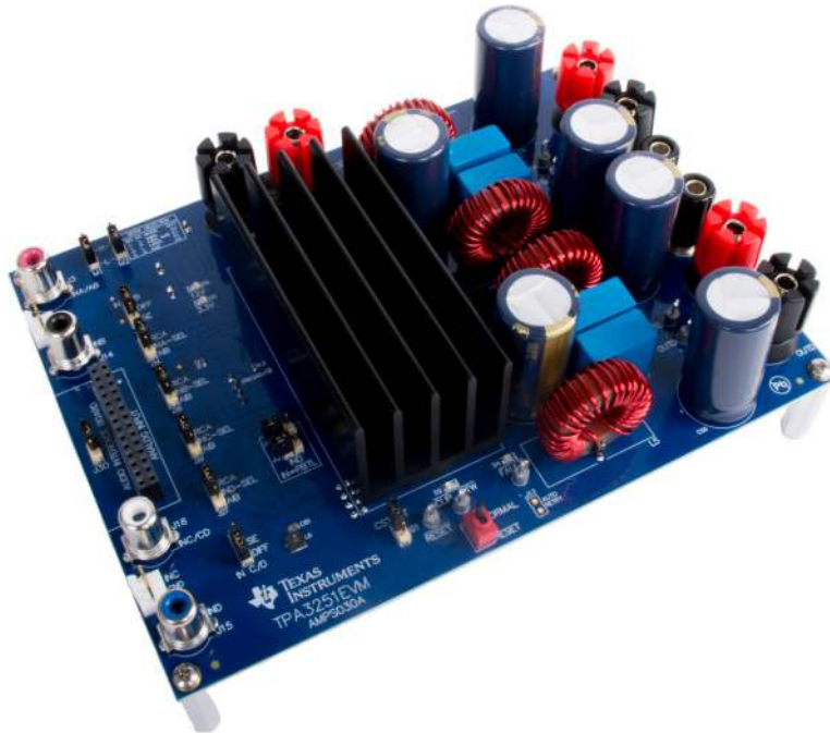
Figure 1. TPA3251 Evaluation Module
