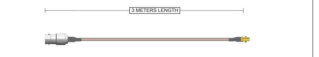
Connector A 112631 BNC Jack Straight Brass Nickel + Heatshrink 50 Ohm RG-178 Continuity/Hi-Pot Connector B 252167 MCX Jack Straight Bulkhead - Rear Mount Brass Gold + Heatshrink
