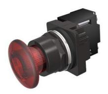
30mm BlackMax, Epoxy Coated Corrosion Resistant Complete Metal Unit Illuminated Push-Pull Operator Full Voltage, 120V AC/DC LED Lamp Mushroom Head Cap Small 1 3/4" (44.5 mm) Plastic, Red 2 Position Maintained, Pull-to-Release UL Listed, CSA Certified NEMA 1,3,3R,4,4X,12,13 & Automotive Standards
