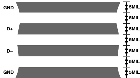
Figure 16. Arrangements of Signal Tracks
