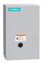
Non-reversing contactor, Size 2 1/2, Three phase full voltage, Contactor amp rating 60A, 3 wire (NO aux included), 110-120/220-240VAC 60Hz coil, Non-combination type, Enclosure NEMA type 1, Indoor general purpose use, Standard width enclosure
