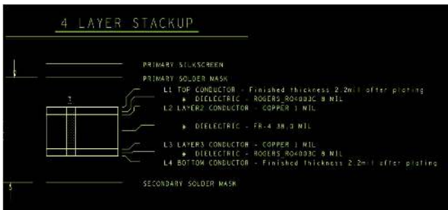
Figure 14. EVAL-ADGM1001SDZ Board Stackup
