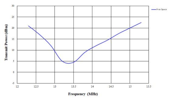
\*HF sensitivity shown in the figure is measured by Voyantic Tagformance HF Loop Antenna C60. Actual sensitivity performance is subject to the environment in practice.
