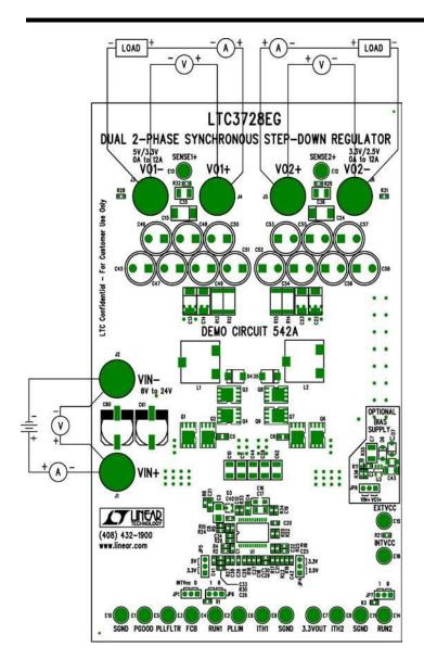
Figure 1. Setup for measurement equipment.
