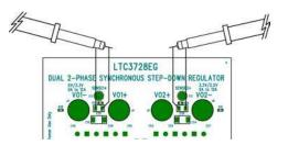
Figure 2. Output ripple measurement.
