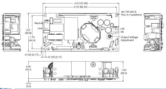
Pin 3 Neutral Mates with JST housing VHR-3N and JST Series SVH-21T-P1.1 crimp terminals
