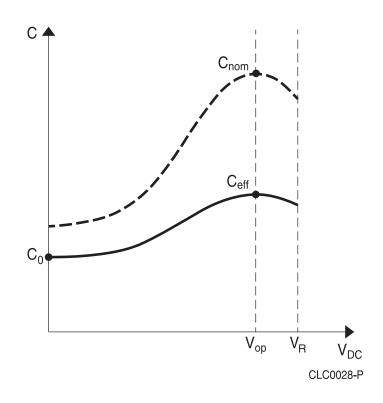
Initial capacitance C<sub>0</sub>: Is the value at the origin of the hysteresis without any applied direct voltage.
