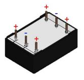
Note that polarity is only for incoming inspection purposes, and it does not affect operation. If put under reverse rated voltage  $V_R$ , CeraLink<sup>®</sup> is repoled and works identically, see our <u>CeraLink</u> <u>Technical Guide</u> for further details.
