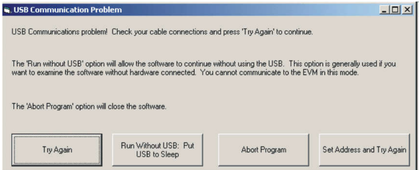
Figure 4-2. INA220EVM Software—No Communication with the USB DIG Platform
