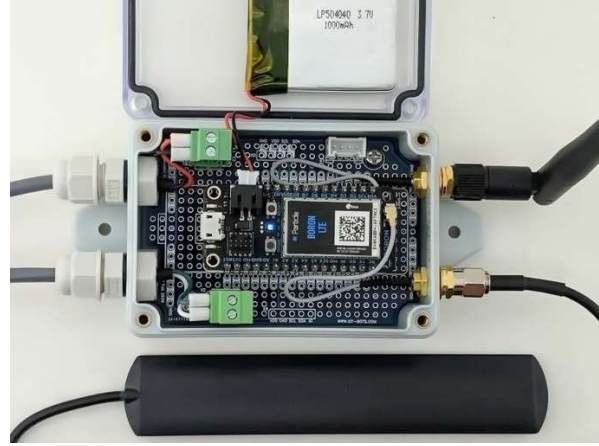
Pic. 19. LiPol battery applied to a transparent lid (inside view)
