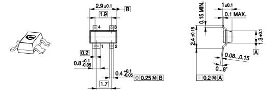
Note: Mold flash, protrusions or gate burrs of 0,2 mm max. per side are not included
