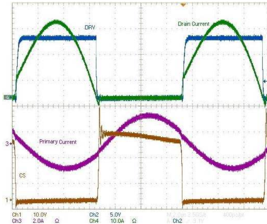
Figure 42. Waveforms from SR System Implemented in LLC Application and Using MOSFET in SMT Package with Minimized Parasitic Inductance – SR MOSFET Channel Conduction Time is Optimized
