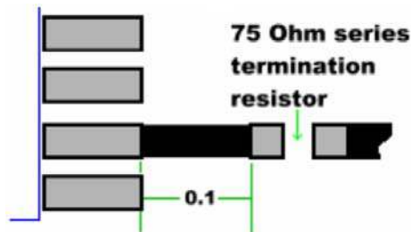
Figure 4. 75\Omega Series Resistor 0.1 Inches from Pin
