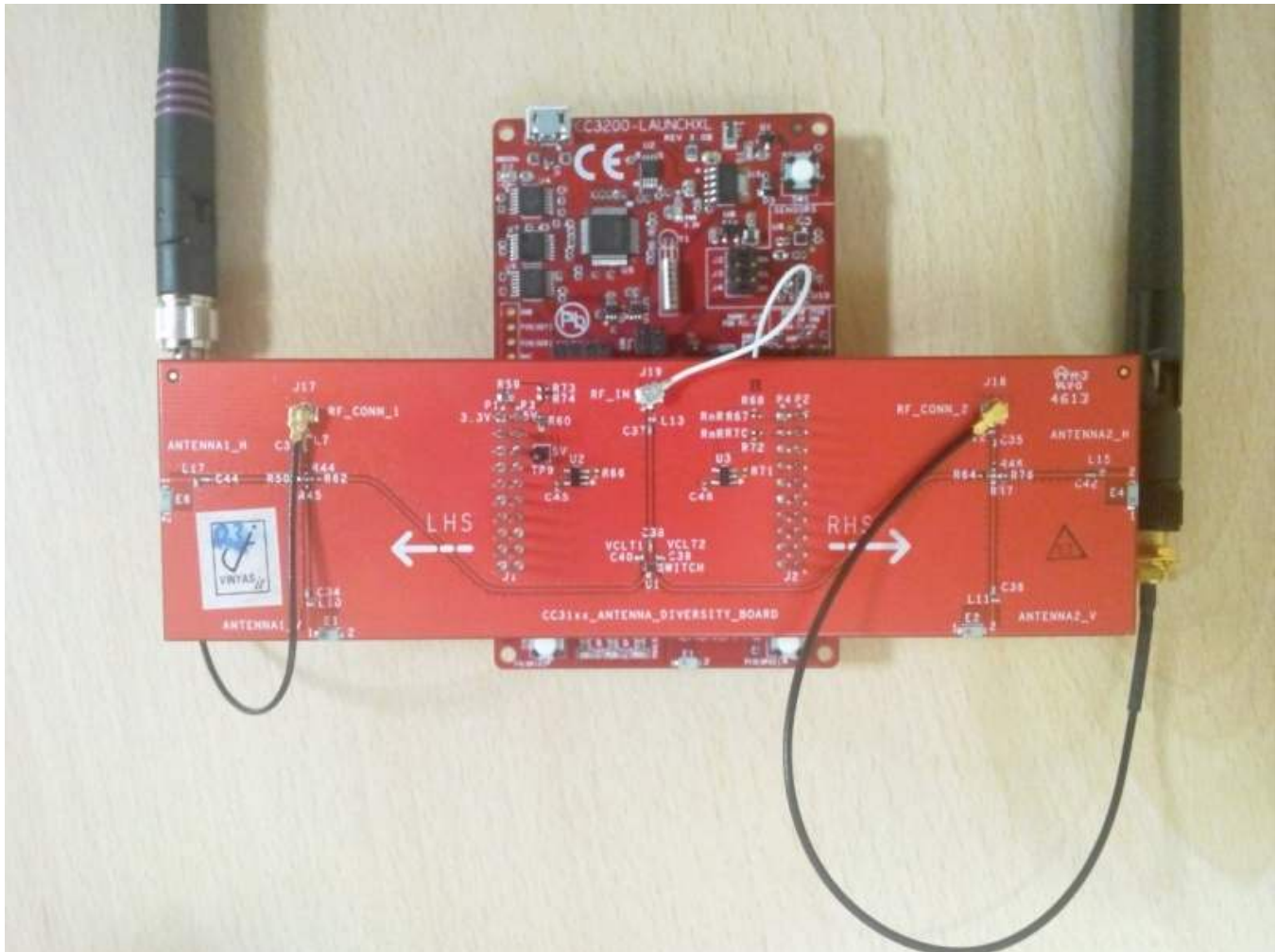
Figure 3-3. Correctly Connected CC3200-LAUNCHXL and CC3ANTENNABOOST Boards
