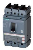
circuit breaker 3VA5 UL frame 250 breaking capacity class H 65kA @ 480 V 3-pole, line protection TM210, FTFM, In=70A overload protection Ir=70A fixed short-circuit protection Ii=10 x In UL489 SB (naval), 50 deg. cel. nut keeper kit on both sides
