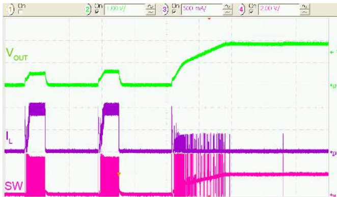
Figure 37. Overload Recovery to Light Load, 50\ \mu\text{s}/\text{div.}
