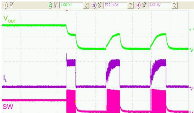
Figure 35. Over-Current Fault Response, R_{LOAD} = 1\ \Omega , 50\ \mu\text{s}/\text{div.}
