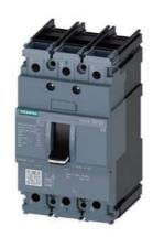
circuit breaker 3VA5 UL frame 125 breaking capacity class M 35kA @ 480 V 3-pole, line protection TM210, FTFM, In=110A overload protection Ir=110A fixed short-circuit protection Ii=10 x In UL489 SB (naval), 50 deg. cel. nut keeper kit on both sides
