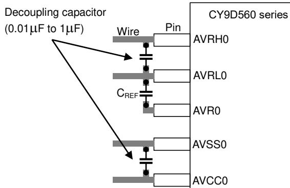
It should be used smoothing capacitor for between AVR1 to AVRL1, RVR0 to RVRL0, RVR1 to RVRL1 as well.
