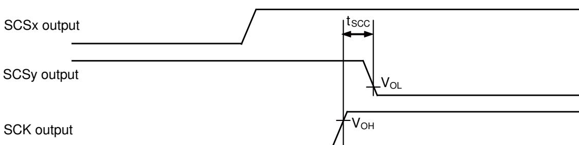
Clock switching example by master mode round operation
