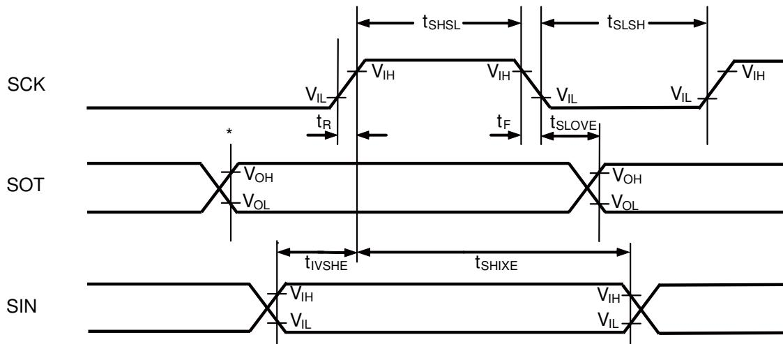
When the Serial Chip Select is Used (SCSCR: CSEN = 1)
