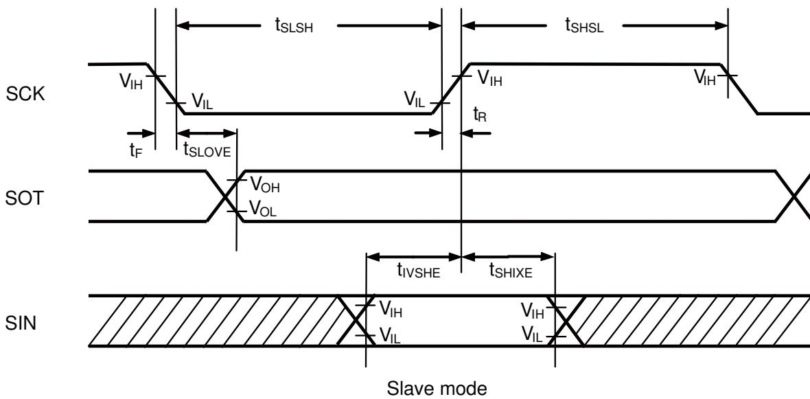
Normal Synchronous Transfer (SCR: SPI = 0) and Serial Clock Output Signal Detect Level "L" (SMR: SCINV = 1)
