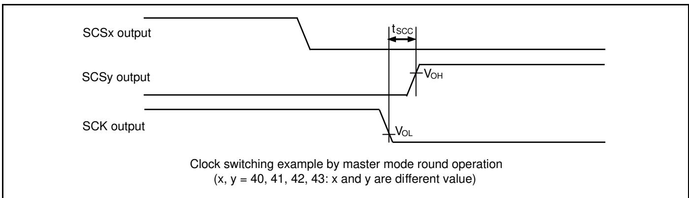
When the Serial Chip Select is Used (SCSCR: CSEN = 1)
