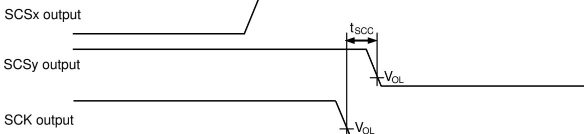
Clock switching example by master mode round operation
