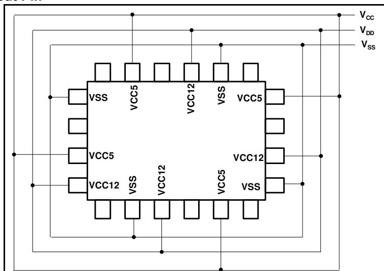
The power supply pins should be connected to VCC5, VCC12 and VSS of this device at the low impedance from the power supply source.
