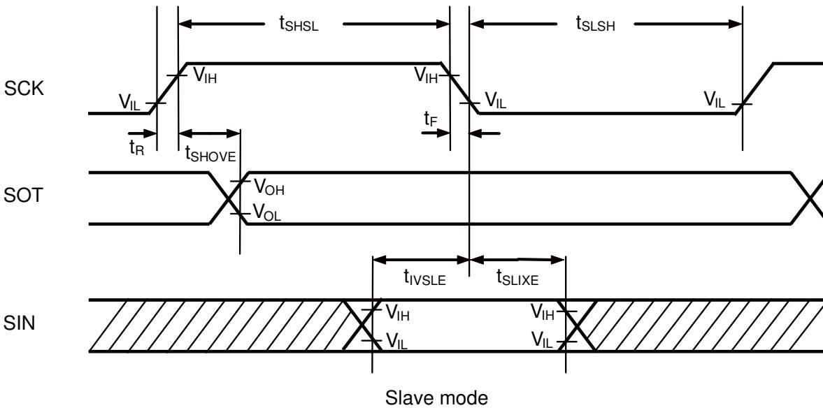
SPI Compatible (SCR: SPI = 1) and Serial Clock Output Signal Detect Level "H" (SMR: SCINV = 0)
