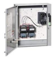
2-speed 3-phase motor starter, Size 2 1/2, Two separate windings, Constant horsepower, Solid-state overload relays, Low Spd OLR range 25-100A, High Spd OLR range 25-100A, 110V 50Hz / 120V 60Hz coil, Combination type, 100A circuit breaker, Enclosure NEMA type 4/12, Water/dust tight for outdoors
