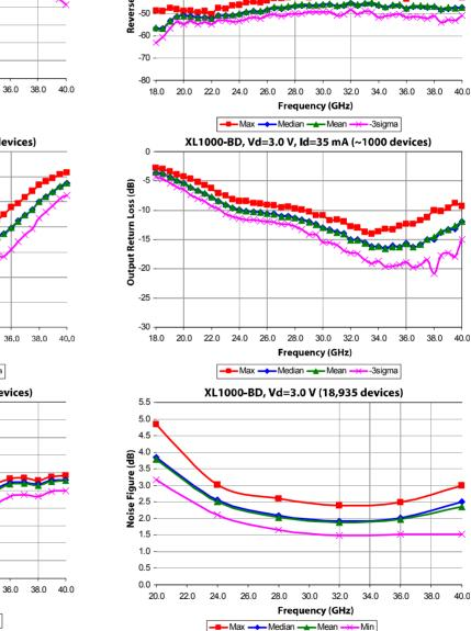
Note [1] Measurements - On-Wafer data has been taken using bias conditions as shown. Measurements are referenced 150 um in from RF In/Out pad edge. For optimum performance M/A-COM-Tech T-pad transition is recommended. For additional information see the M/A-COM-Tech "T-Pad Transition" application note.
