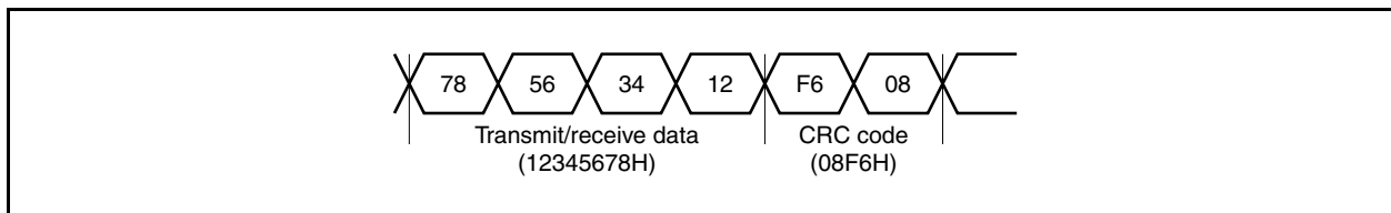
Figure 25-4. CRC Transmission Example
